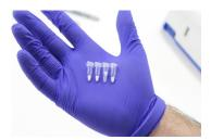
Reaction Pellets are light sensitive. Immediately place remaining reaction pellets back into the desiccated tube and then insert the desiccant tube into the foil pouch to protect from light.
