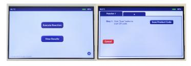
**2.** Scan the barcode found by following the hyperlink on page 1. The barcode scanner is located on the left side of the AmpliFire.
