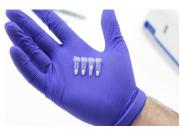
Reaction Pellets are light sensitive. Immediately place remaining reaction pellets back into the desiccated tube and then insert the desiccant tube into the foil pouch to protect from light. **5.** Transfer  $25 \mu$  from the colored tube containing your sample extract into the reaction pellet (clear tube).
