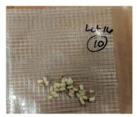
**2.** Extract with GEB extraction buffer at a ratio of 1:10 (w:v) in a mesh extraction bag (0.3 g/3 mL). Let rest for 5 minutes at room temperature.
