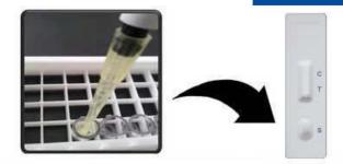
Take out microwells from package,use Pipette absorb 150ul sample into microwell, beat and blow evenly, then transfer all liquid into "S" well on test card, be static for 5-8min, read the result.
